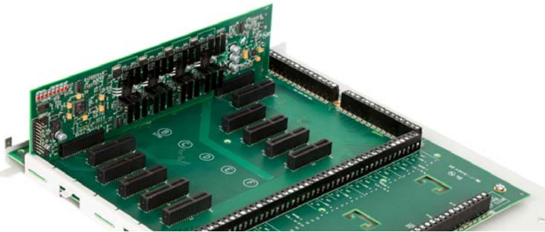
Figure 2-25 Secure Position for Circuit Boards in the Chassis
