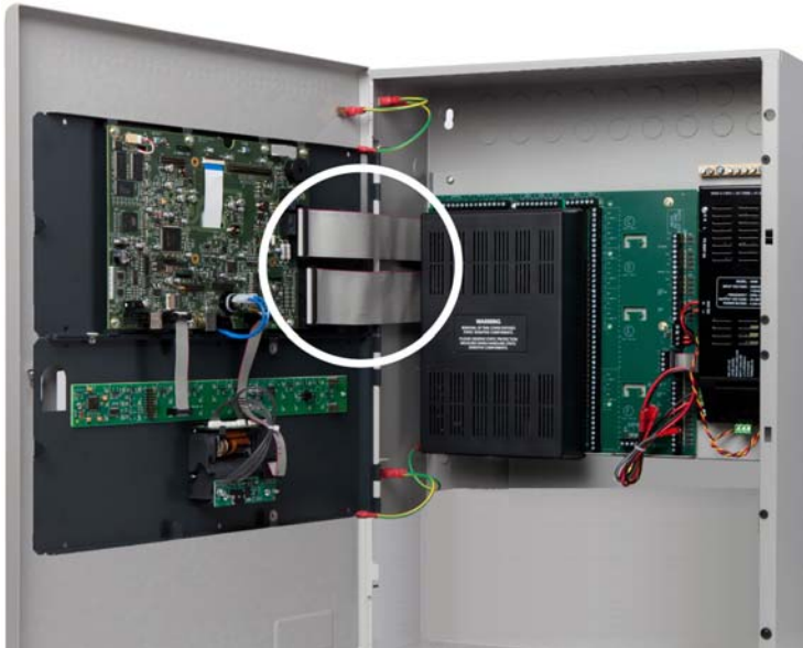
Figure 3-8 Removing Ribbon Cables
