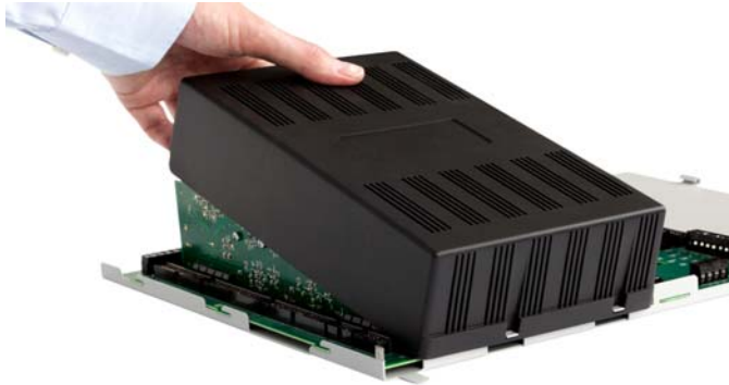
Figure 2-23 Removing the Chassis Cover
