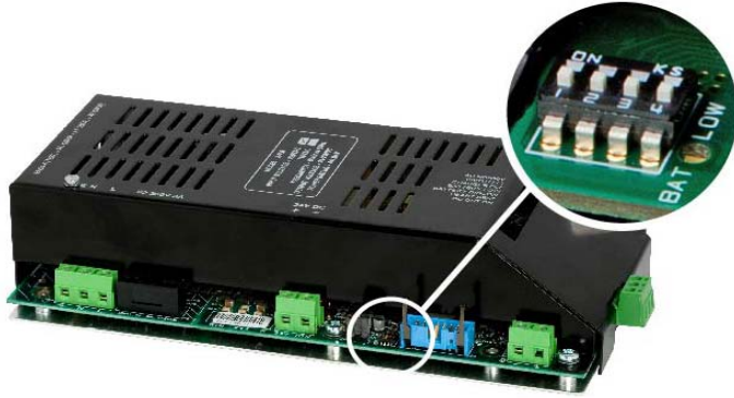
Figure 2-17 Dip Switch Position
