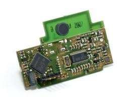
Wireless module for smoke detector HDv 3000 0 (No. 30458) for wireless transmission of alarms and fault messages to the wireless fire control panel RCP 6B:
