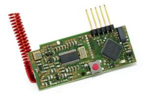
Update module to equip thermal home detector TM (No. 31957) with, for wireless transmission of alarms and fault messages to the wireless fire control panel RCP 6B:
