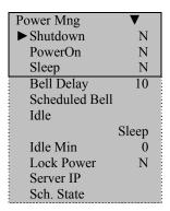
The B&W screen FRT adopts an intelligent power management system and supports such functions as timing power-on/shutdown and sleep timing.
