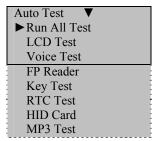
Through this menu, you can test the system components. The auto test function helps troubleshoot the FRT quickly and facilitates the FRT maintenance.
