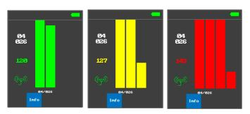
The screen will display graphs of received signal level, the number and color of which varies, depending on the signal level when approaching or moving away from the signal source (video camera).
