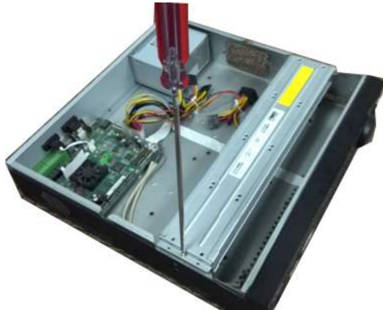
Figure 3-36 Open the top cover
