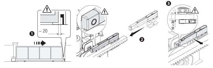
Fasten the support to the rack using the grub screws supplied.
