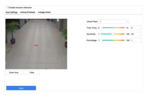
**Figure 5-6 Intrusion Detection**
