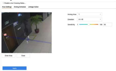
**Figure 5-7 Line Crossing Detection**
