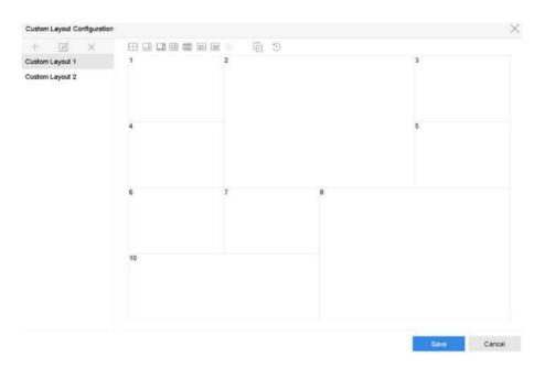
Figure 3-2 Configure Live View Layout
