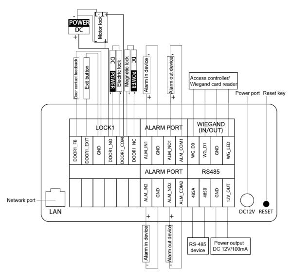
Figure 2-1 Cable connection
