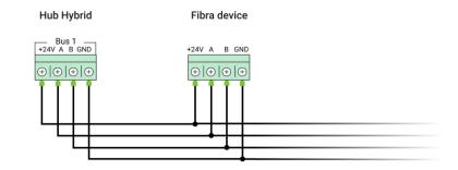
+24V — power supply input A, B — signal terminals GND — ground
