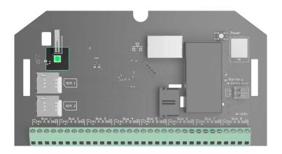
Depending on the state of communication between the control panel and the Ajax Cloud server, the Hub Hybrid LED indicator lights up in three colours: white, red, or green.
