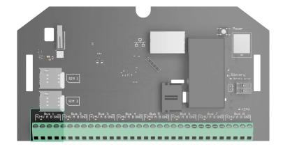
Hub Hybrid (2G) / (4G) has 8 buses. Numbers from 1 to 8 are indicated on the control panel board.
