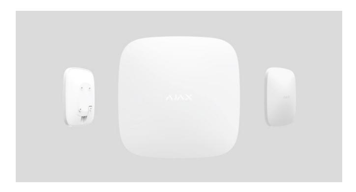
**Hub** is a central device of the Ajax security system, coordinating the connected devices, and interacting with the user and security company. Hub is developed only for indoor use.
