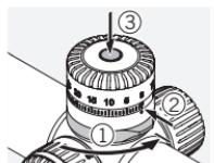
Open the locking mechanism on the turret. **Check the zero position.** Using a pointed object, press in the middle of the turret.
