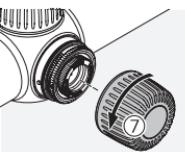
Remove the screw-on cap on the side turret of the scope.
