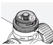
Put the marking rings on the turret on the basis of the information in the ballistic program and align them with the index point.
