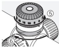
Now you can choose the settings you want on the turret. Rotate the locking mechanism one quarter turn clockwise to lock it.
