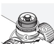
Open the locking mechanism on the turret. Turn the marking on the turret to zero if it has moved to another position.
