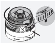
Turn the turret 35 clicks counter-clockwise and align the >|< marking on the top of the scale with the index point. Then close the locking mechanism.
