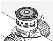
Check the zero setting of the turret and lock the locking mechanism. Unscrew the knurled ring from the turret.
