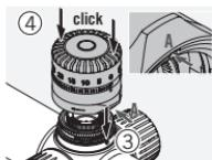
Install the turret to the scope until you hear a click. Note the zero position while doing this.
