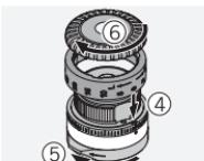
Install the right/left graduated ring. Make sure that the zero is aligned with the index point. Close the locking mechanism. Screw the knurled ring back onto the turret.
