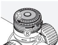
Once you have put the marking rings on the turret, screw the knurled ring back on.
