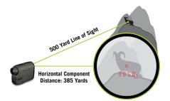
The displayed HCD yardage is corrected for shot angle and needs no extra user input; shooters simply use the appropriate level ground bullet drop for the range displayed. Archers use the appropriate level ground sight pin for the range displayed.
