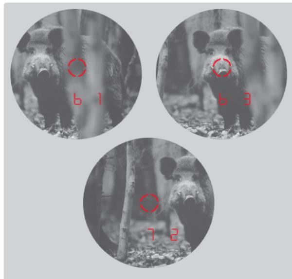
The Leica Rangemaster can also be used for continuous measurements (scan mode): Press and hold the main button **2** when it is activated a second time. The device switches to scan mode after about 2.5 s and will then measure continuously. Scan mode is indicated by a change in the display. A new measured value appears every 0.5 s.
