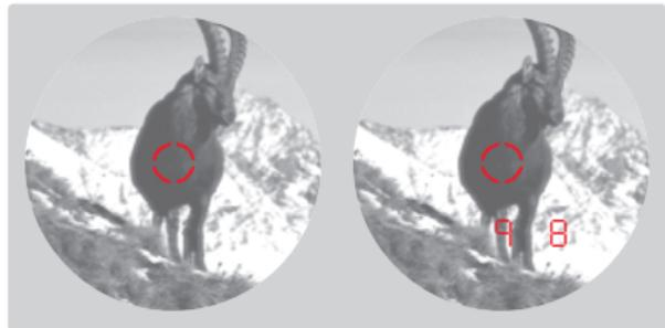
Aim directly at an object to measure its distance. Proceed as follows:
