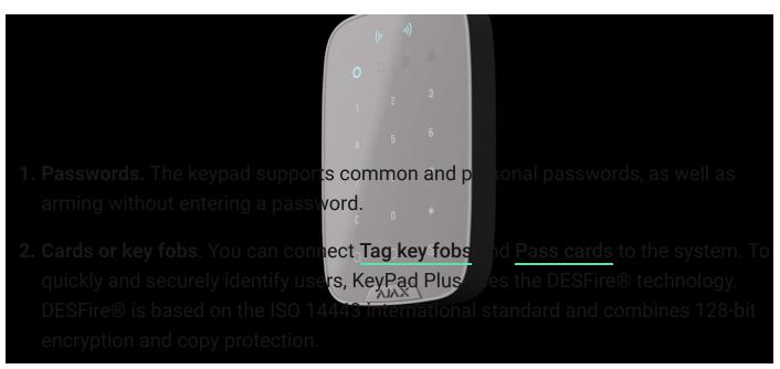
Before entering a password or using Tag/Pass, you should activate ("wake up") the KeyPad Plus by sliding your hand over the touch panel from top to bottom. When it is activated, the button backlight is enabled, and the keypad beeps.
