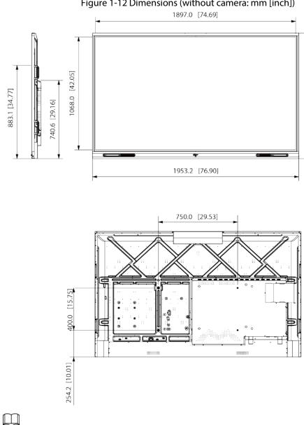
Figure 1-12 Dimensions (without camera: mm [inch])
