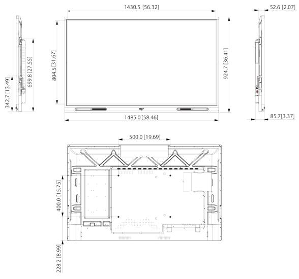
Figure 1-8 Dimensions (without camera: mm [inch])
