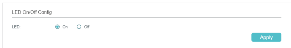
Figure 2-8 Configuring LED On/Off
