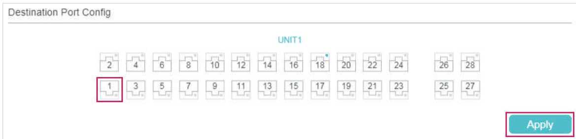
Figure 2-3 Destination Port Configuration
