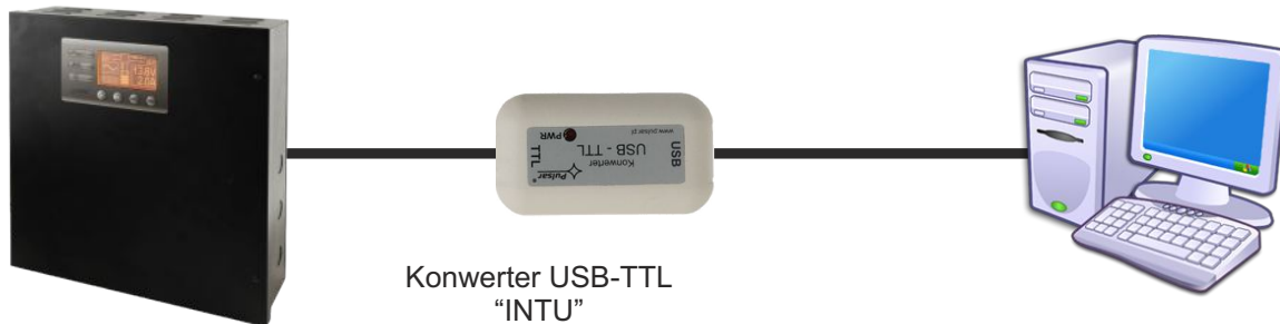
USB-TTL communication using the USB-TTL „INTU” interface.
