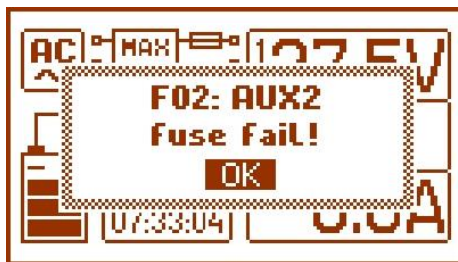
Fig. 11. Message indicating blown fuse at the AUX2 output.
