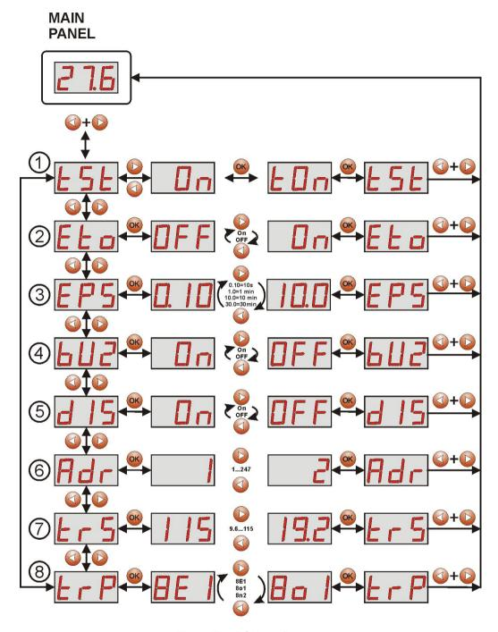
Fig. 9. The PSU configuration menu.
