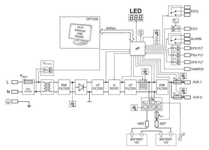
Fig. 1. PSU block diagram.
