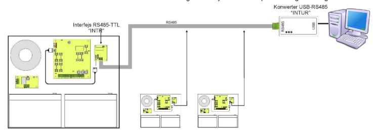
Fig. 20. RS485 communication using the "INTR" and "INTUR" interfaces.
