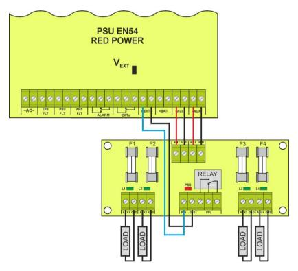
Fig.14. The connection of fuse module.
