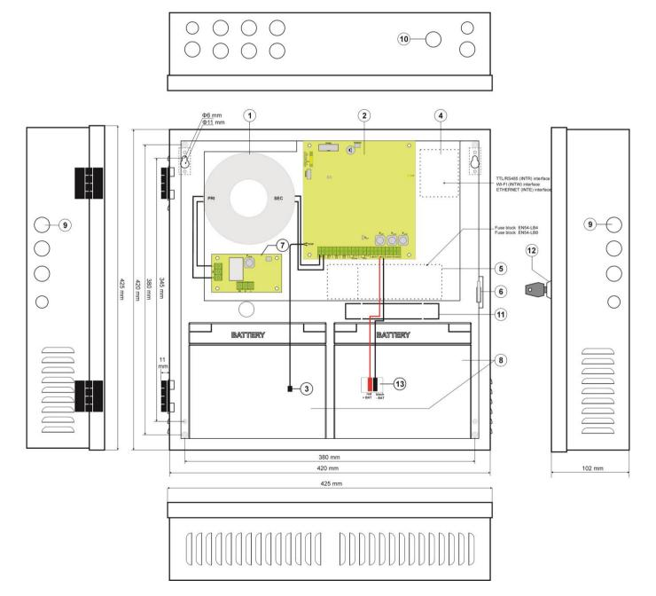
Fig.4. The view of the PSU.
