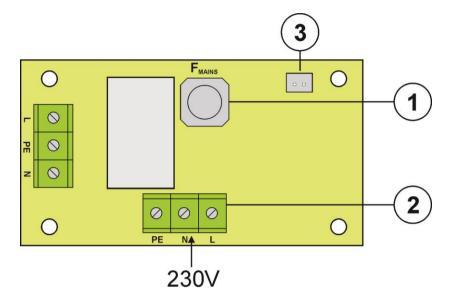
Fig. 3. The view of the EMC filter.
