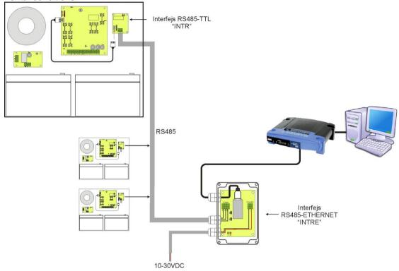
Fig. 17. Ethernet network communication using the RS485 "INTRE" interface.
