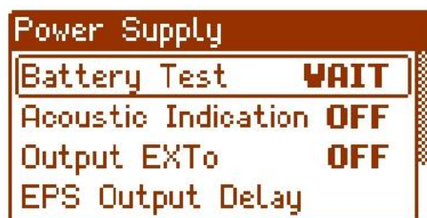
Fig. 27. Temporary lock of the battery test.
