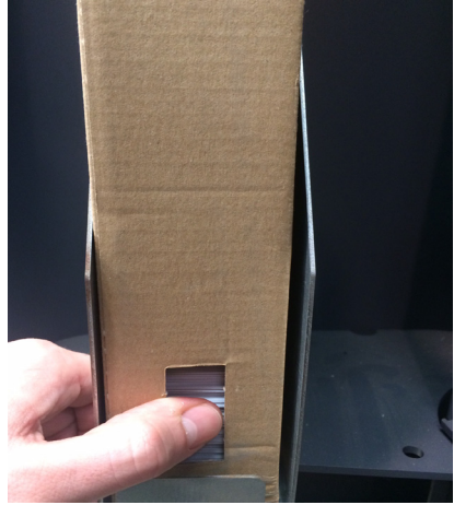
6 - For the paper sensor to work correctly, push the tickets from the packet window.
