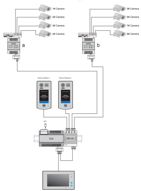
NOTE: The system can connect SC6V, but at this time, the DIP6 of DT-QSW must be set to ON.
