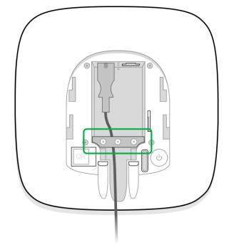
**4.** Slide ReX 2 onto the mounting panel. After installation, check the tamper status in the Ajax app and then the quality of the panel fixation. You will receive a notification if an attempt is made to tear the range extender off the surface or remove it from the mounting panel.
