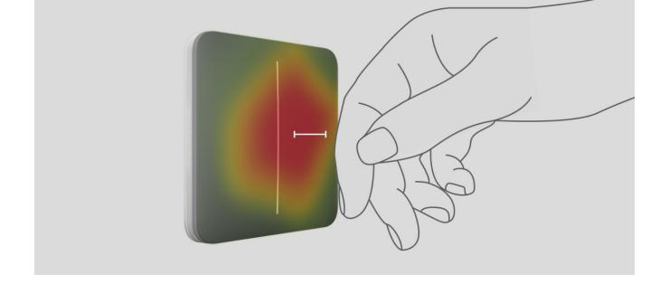
LightSwitch allows controlling lighting when a hand is 15 millimetres away from the switch or when touching the touch-sensitive panel of the switch. Contactless control does not limit the possibility of use, even if hands are dirty or wet. The sensor reacts under any conditions. Therefore, the switch can be installed in crowded places: restaurants, factories, and offices.
