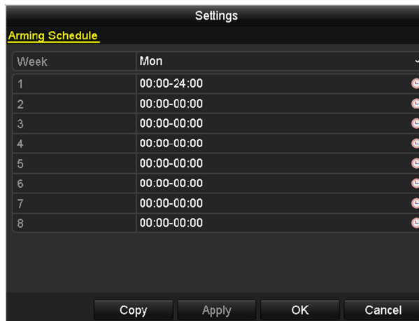
Figure 10-16 Set Arming Schedule of Alarm Output
