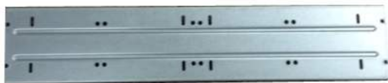
Figure 3-37 Take out HDD bracket
