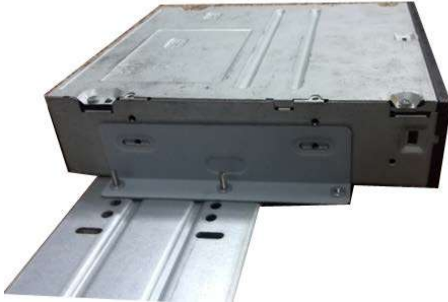
Figure 3-43 Install SATA burner
