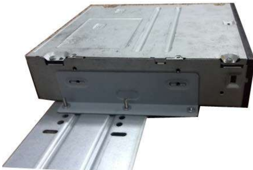
Figure 3-43 Install SATA burner
