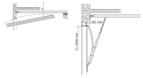
For protracting, partially retracting overhead doors, use the V201 transmission arm (optional accessory).
