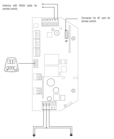
OPEN-CLOSE-INVERT (step-by-step) function from control device (NO contact). Alternatively, from function programming you can activate other commands. See function F 7. STOP button (NC contact). Enables the door to stop and excludes the automatic closing. To resume movement press the control button or use another control device. See function F 1.
