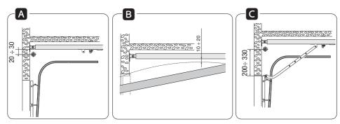
For protracting overhead doors, keep the guide 20 mm from the opening high-point.
