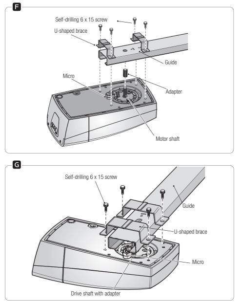
$\triangle$  If the operator is to be fitted at a right angle, before installing it, set the micro-switch (see the corresponding paragraph).
