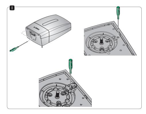
Perforate the cable gland ① pass the cables through ② and fit it into its corresponding housing ③. □ The number of cables depends on the type of system and accessories fitted.
