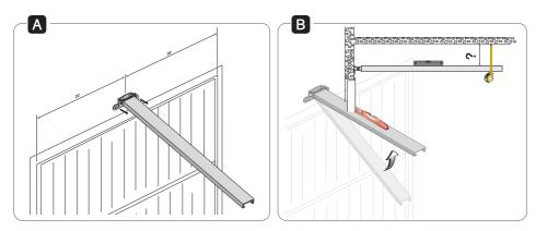
Bend the perforated flat tabs so they fit snugly and so as to compensate for the distance between the guide and ceiling.
