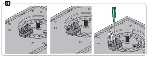
Remove the operator's cover. Pull out the electrical cable and fit it through the hole.
