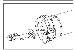
Loosen the screw to remove the support square shaft.
