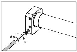
A - Rotate the crank in the direction A to close.
