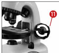
Adjust the microscope stage (7) so that it goes all the way down to the lowest position (11). Then, turn the objective
