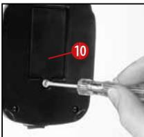
In the base of the microscope there is a battery compartment (10). Loosen the screw at the battery compartment cover with a small Philips screwdriver and re-
