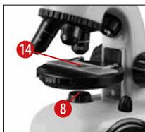
Now place the prepared specimen (14) directly under the objective on the microscope stage. The object should be located directly over the illumination (8).
