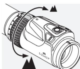
You can set the desired magnification by turning the (stepless) magnification adjustment ring through 180°. The scale on the adjustment ring allows simple and easy reading of the setting.
