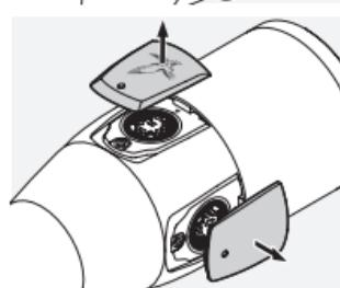
3. Elevation adjustment: Turn the adjusting tool in the middle of the elevation adjustment...
