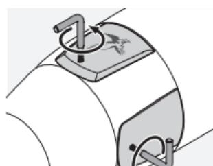
2. The covers of the elevation and windage adjustment can be opened with the provided torx wrench (TX 6). You can then adjust the elevation and windage adjustment when open with the adjusting tool.
