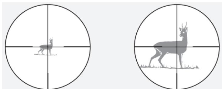
If the magnification increases, then the reticle remains the same size - the size of the image is increased but not the size of the reticle and the display. Even for large magnifications only a little of the target is covered.
