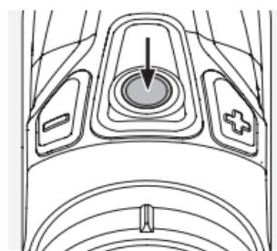
An illuminated circle, the aiming mark for distance measurement, appears after you press the measurement button and the measuring function is activated. If you release the measurement button,
