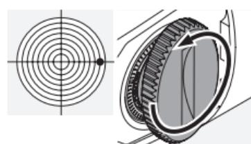
b) ... counterclockwise for a shot to the right for the required impact point correction (per click 1/4 MOA; 7 mm/100 m or 0,25 in/100 yds).
