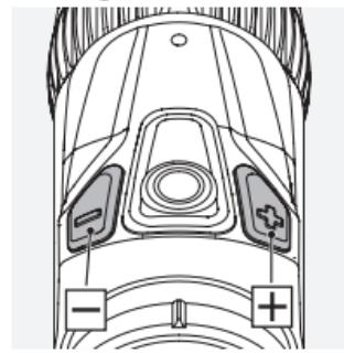
Once the reticle illumination is turned on, you can now adjust the brightness by means of the +/- buttons and select the setting of your choice from among 64 brightness levels. Keep the button pressed (constant impulse) to rapidly find the optimum brightness, to adjust finely press the button once (single impulse).
