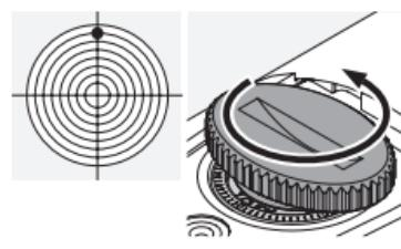
b) ... counterclockwise if the shot is high for the required impact point correction (per click 1/4 MOA; 7 mm/100 m or 0,25 in/100 yds).
