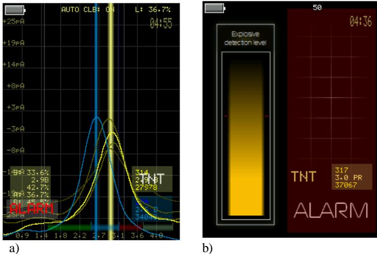
Figure 21. Weak signal for explosive vapors.
