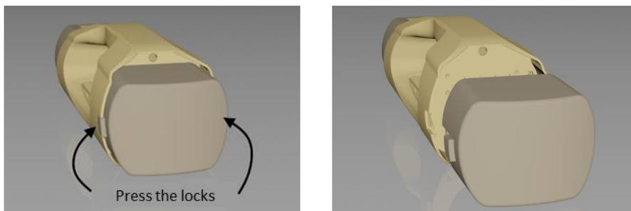
*Figure 22. Battery unit replacement*
