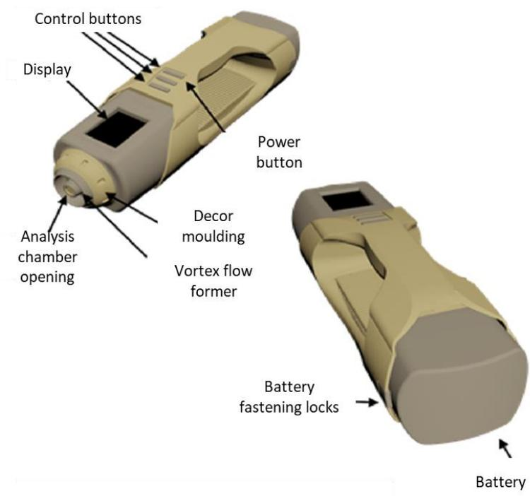
Figure 2. Location of control buttons and indicator
