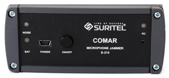
NOISE – indicator of turning the noise interference.
