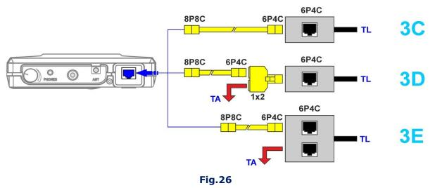
Ways of **parallel-connecting** to telephone lines, when end user devices (telephones or facsimile machines) need to be in operation, are shown in fig.26, **3D and 3E**.
