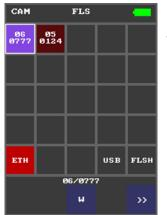
To move the cameras to the "white" list from the home screen, first touch the selected cell with your finger or stylus (it is highlighted with a white border), and then click on the **"W"** button – the cell with information automatically moves to the second page of the screen and turns green.
