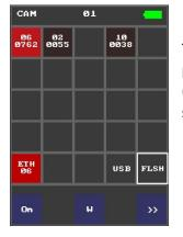
To search and localize the detected video camera press the cell and hold for two seconds, then a scale (column) with the signal level will appear on the screen.
