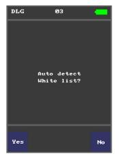
The device provides a mode for automatically transferring all currently detected signals to the "white" list. To do this, on the main screen, without selecting a specific cell, press the **"W"** button. You will be asked to start the automatic detection mode and transfer signals to the "white" list.
