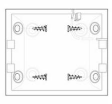
1. Attach the SmartBracket panel to the surface using bundled screws, using at least two fixing points (one of them – above the tamper). If you select other attachment hardware, make sure that they do not damage or deform the panel.
