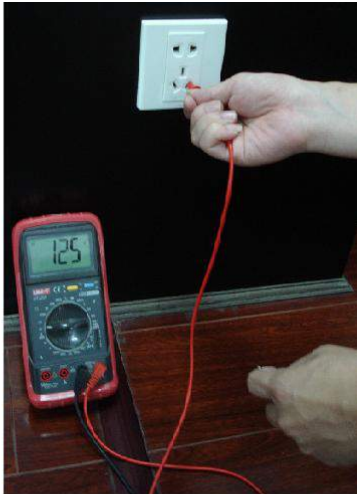
Appendix Figure 7- 6 Check live cable connection
