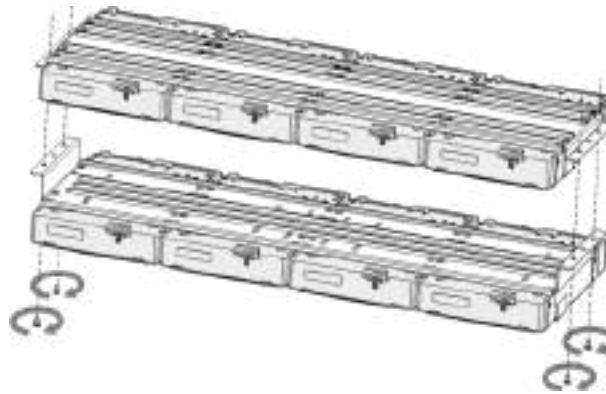
Figure 2-12 Fix drive brackets
