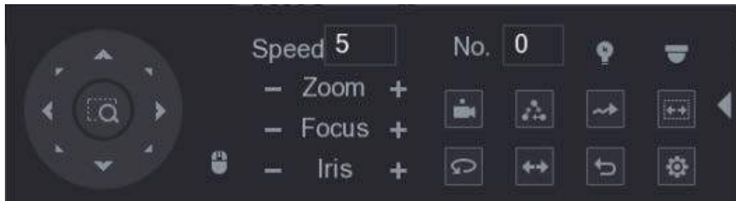
Figure 5-53 Expanded PTZ control panel
