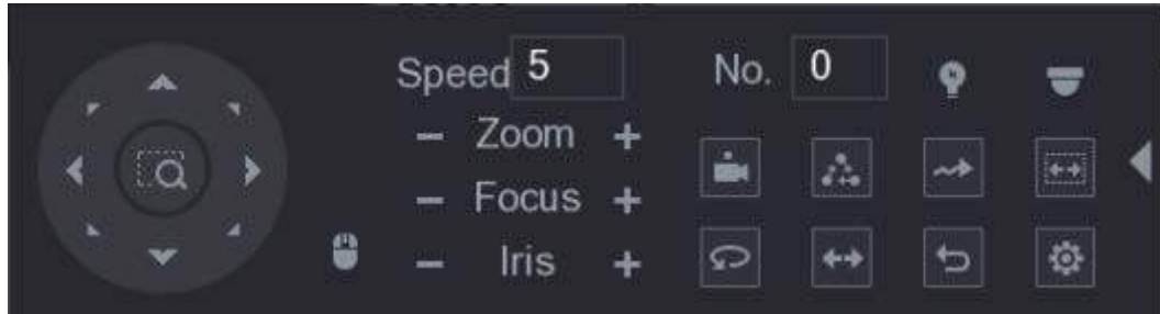
Figure 5-63 Expanded PTZ control panel
