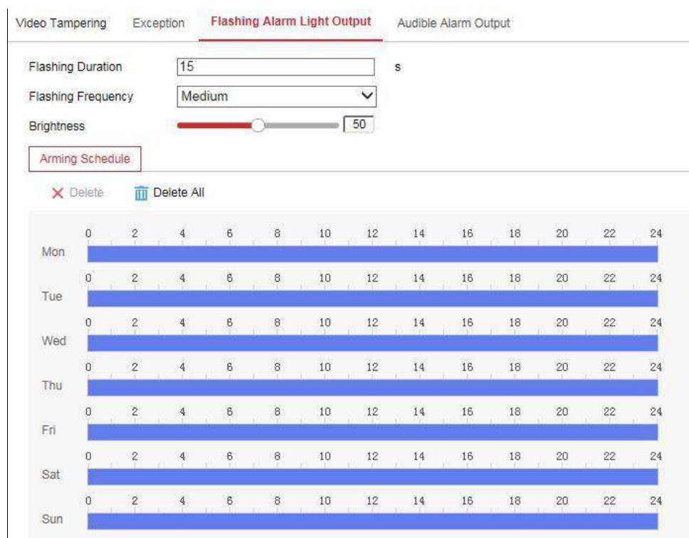
Figure 10-9 Flashing Alarm Light Output Settings
