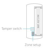
**NOTE:** Tamper will be triggered no matter the door/window contact is armed or disarmed.
