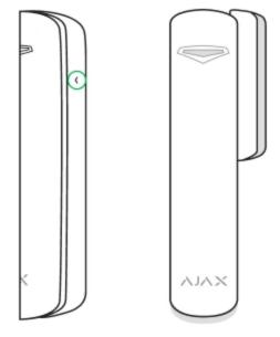
When installing the detector in the perpendicular planes (inside the case/frame), use the small magnet from the set. The distance between the magnet and detector should not exceed 1 cm.
