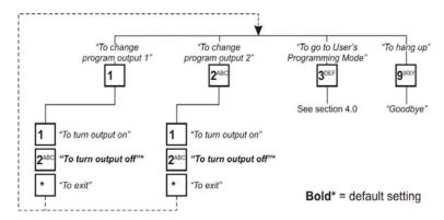
The User's Opening Menu allows you to activate or deactivate the programmable outputs. The programmable outputs (PGM1 & PGM2) can be used for remote switching of other devices. For example, a PGM can be used to turn on air conditioning or heat, extinguish lights, activate a sprinkler system, or open a garage door. Speak to your installer for more information.
