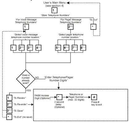
The ParaVox unit can store up to four telephone numbers in locations [1] to [4] and up to four pager numbers in location numbers [5] to [8]. When a telephone number location is assigned to a zone (see *Telephone Number Assignment* on page 13), the ParaVox will dial the number programmed here whenever the zone is triggered. The telephone numbers are programmed into the desired locations as described above.
