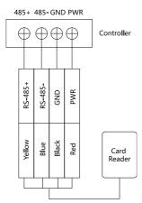
Figure 3-3 Wiring for RS-485 Communication Mode
