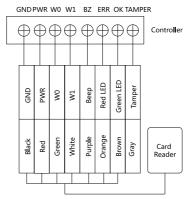
Figure 3-4 Wiring for Wiegand Communication Mode
