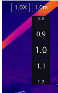
Figure 3-2 Adjust Parallax Correction
