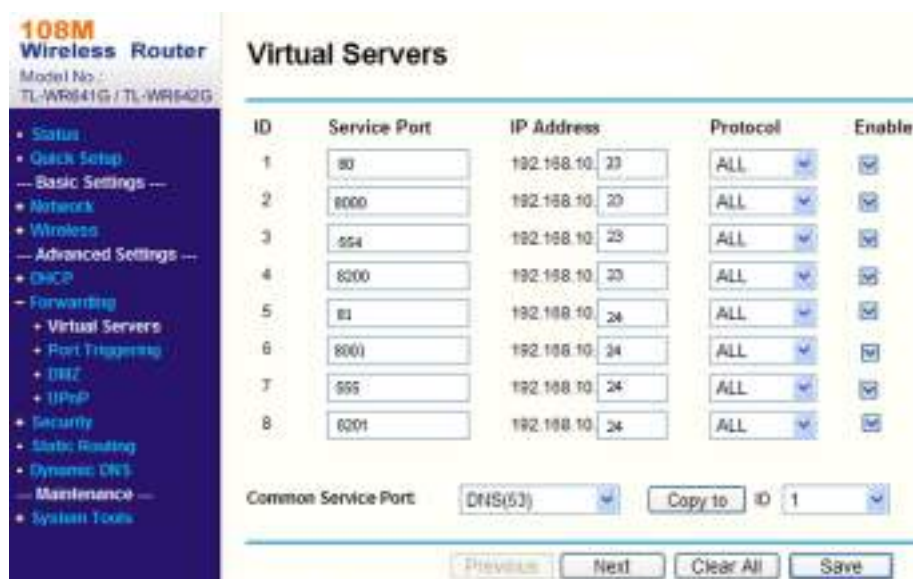
Figure 7-1 Port Mapping on Router
