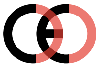
False CE Mark (too close)
