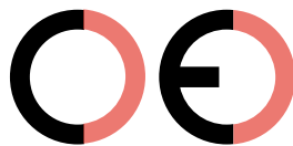
False CE Mark (too far)
