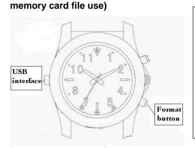
First, press and hold the format button to connect the data cable to the charger or the computer USB interface, this time the blue lights flashing is said to be formatted, when the blue light is bright when the format is completed. Because the memory card format is not right or the file is damaged, it can not be operated, please format it on the machine before it can be used normally.
