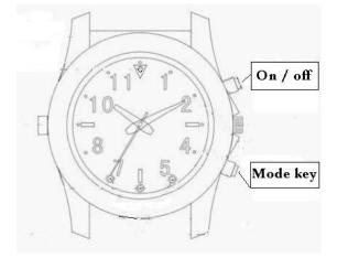
This machine for the combination of key reset, you must press the switch key and boot key, when the machine fails or crash, you can press the two buttons to reset the shutdown.
