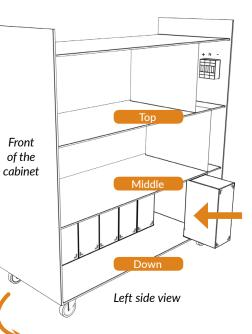
4.2 Then, on the same tray, place another 7 batteries upwards, with the terminals down, this time with the terminals towards the left of the cabinet.
