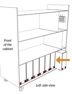
**4.3** Populate middle tray with batteries, sitting upright, first row of 7 batteries with terminals towards the right of the cabinet, but this time placed with the terminals up (as opposed to the tray below).
